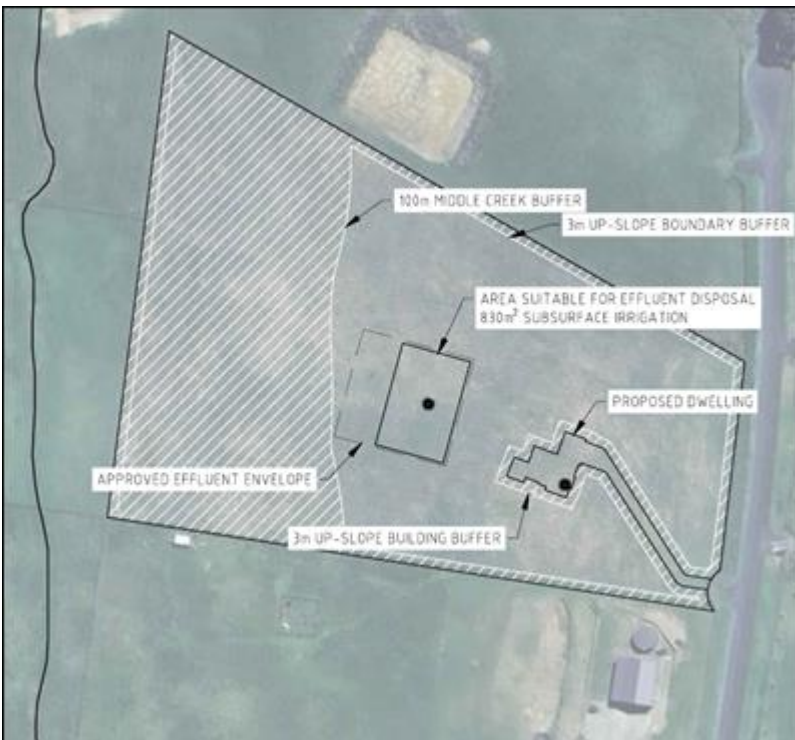
Proposed site plan showing location of dwelling effluent disposal area and 100m buffer from Middle Creek
