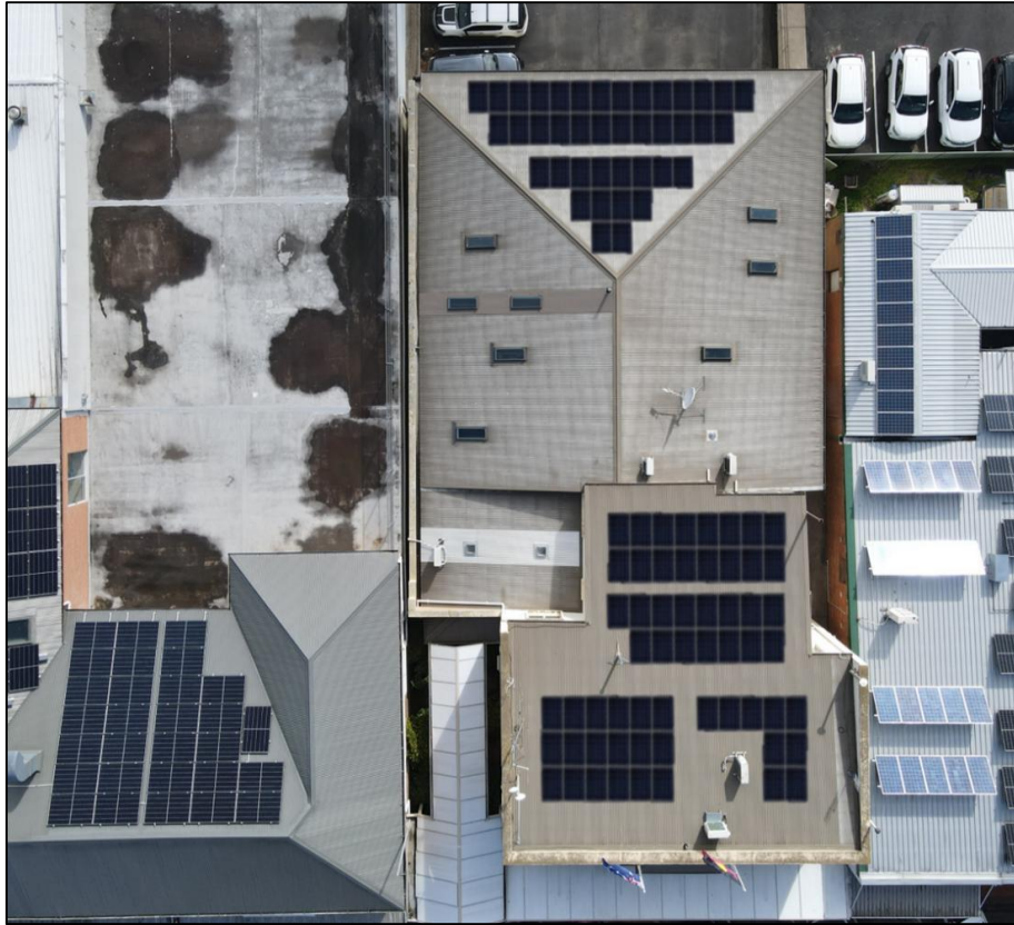
Figure 8: Proposed 37kW roof-mounted solar PV
