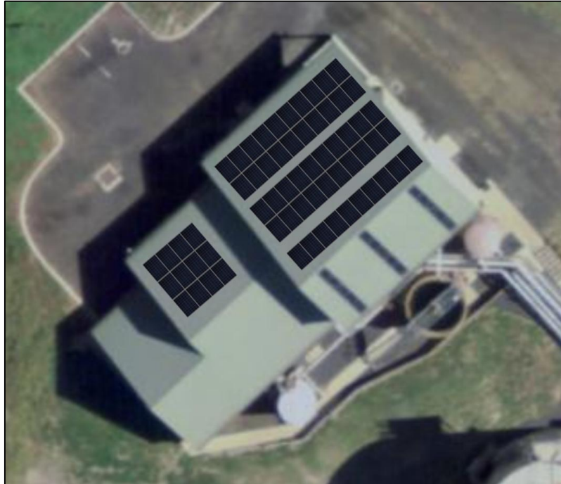
Figure 4: Proposed 30kW roof-mounted solar PV
