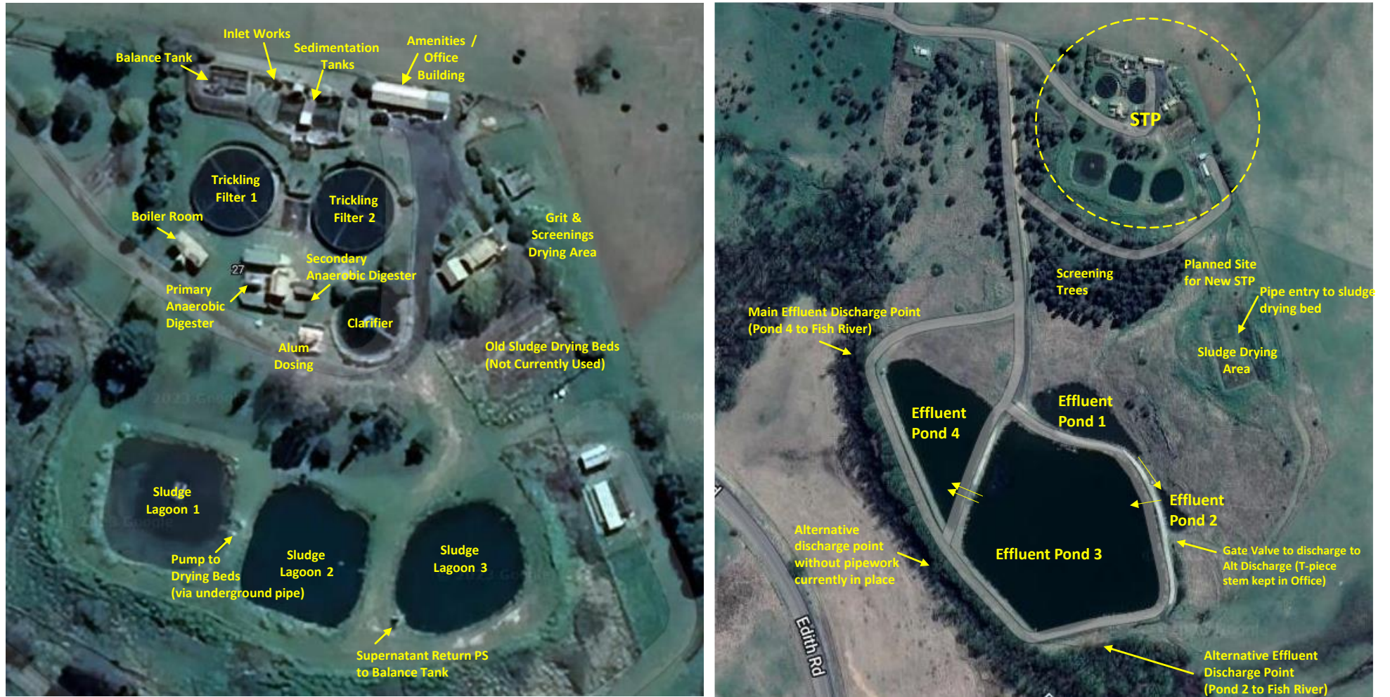
Figure 2-3 Oberon STP Site Layout
